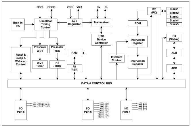
Figure 6-1 EM78612 Series Function Block Diagram
